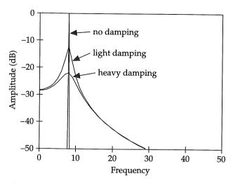
Figure 8.2 Power spectra of the waveforms shown in figure 8.1. Note that increased damping corresponds to wider bandwidth of the spectral peak.
