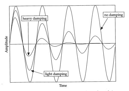
Figure 8.1 An undamped sine wave compared with two damped sine waves identical in frequency and phase.
