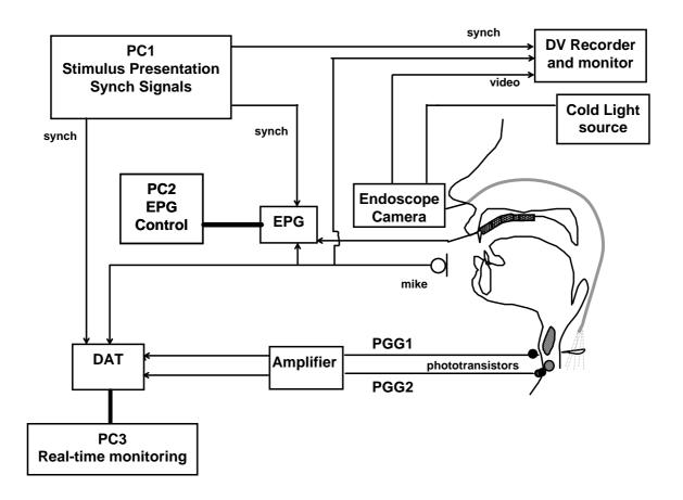
**Fig. 4.1:** Experimental setup for synchronized acquisition of audio, transillumination, electropalatographic and video signals.
