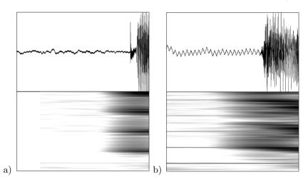
Figure 8: Oscillogram and sonagram of an audiosignal, recorded on a laptop running a) on batteries and b) connected to the power mains. The right oscillogram shows a marked sigsaw-pattern, and the sonagram shows thin horizontal lines at multiples of the mains frequency.
