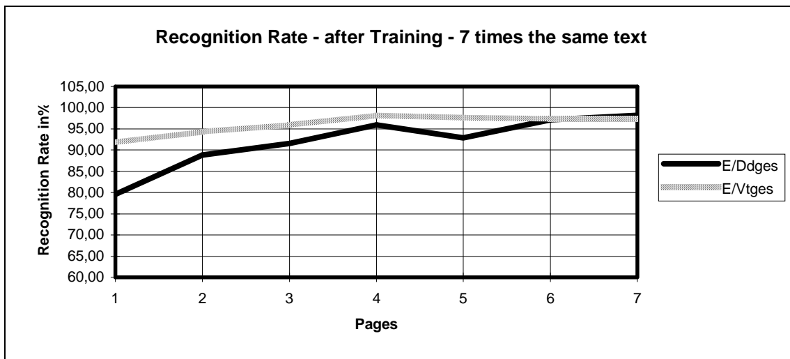
Figure 4: Recognition rate in % after six pages dictation and seven dictations of one and the same page; E/Ddges=Dragon Dictate, E/Vtges= IBM Voice Type
