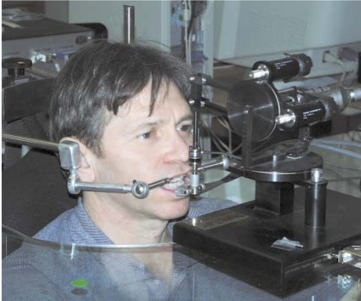
Perturbation of jaw movements using a robotic arm. Image courtesy of David Ostry, McGill University, Montreal, Canada.
