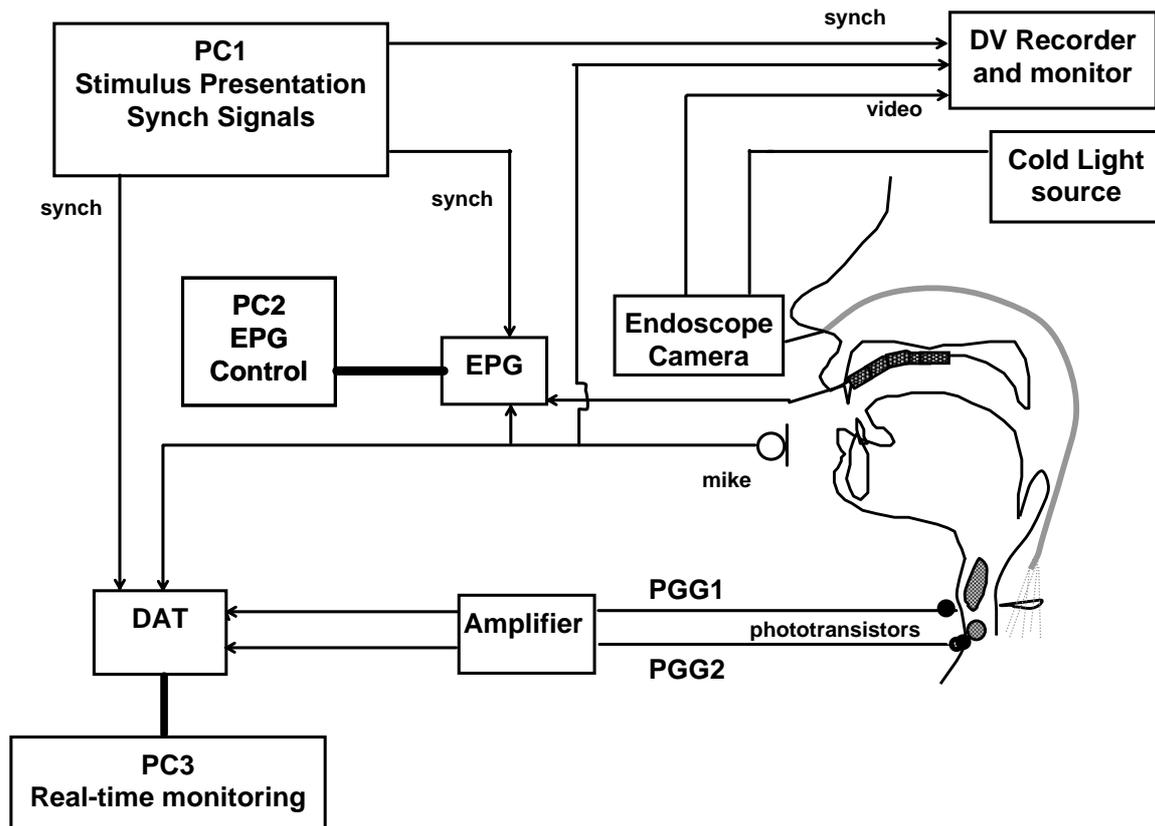
**Fig. 4.1:** Experimental setup for synchronized acquisition of audio, transillumination, electropalatographic and video signals.
