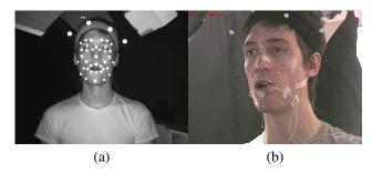
Figure 2: Example still images from the gray scale video from the OptiTrack system (a) and the color video from the camcorder (b).
