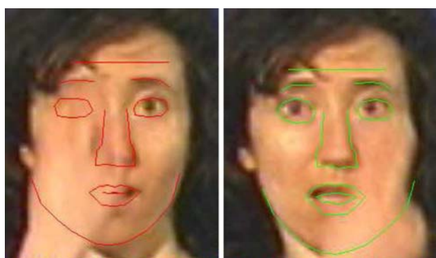
Fig. 32 During the overlapping of the hands and face several regions of the face are evaluated separately. If e.g. mouth and one eye could be hidden ( left ), no features of the face are considered. However, if eyes and mouth are located sufficiently the won features could be used for the classification ( right )
