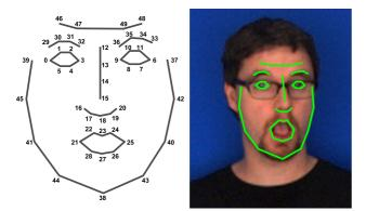
Figure 5. Face graph with 50 landmark points (left) and its application to a specific signer (right).
