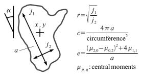
Figure 3. Shape-based features computed for each hand.
