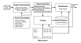
Figure 2. Schematic of the developed sign language recognition system, combining manual and facial features.
