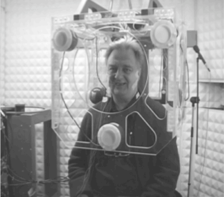
Fig. 5.2. The Carstens Medizinelektronik EMA 'cube' used for recording speech movement data.
